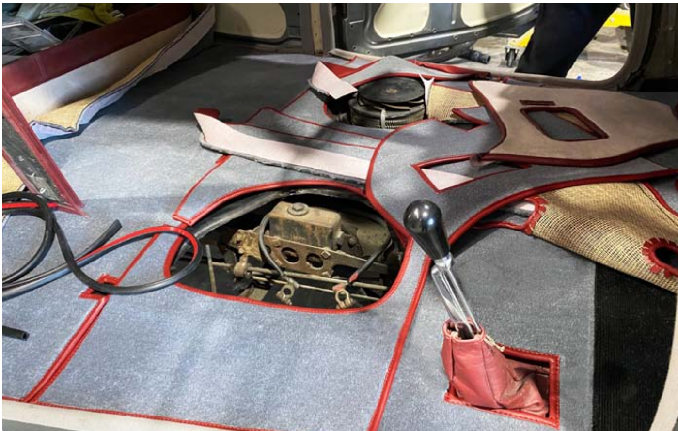
Below: This shot of the new carpet being installed in the Silver Dawn's cabin emphasises the exemplary quality of the work being carried out on this car. Note the brake master cylinder and battery leads visible through the access hatch under the driver's seat, and the heater matrix and fan on the passenger's side.
