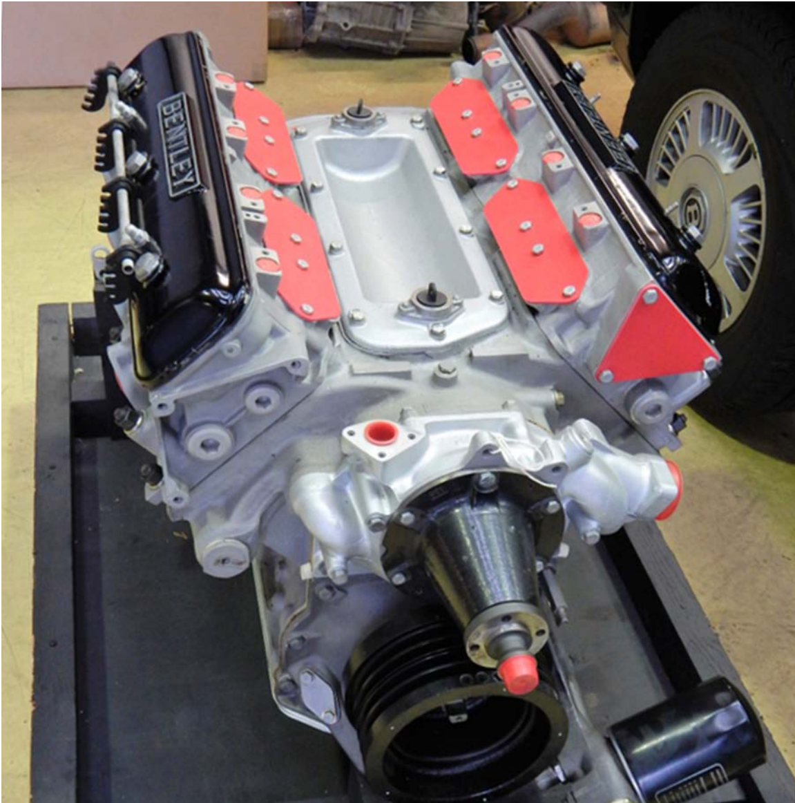
Above: The brand new 6.75-litre V8 engine newly arrived from England, with the car's original Bentley rocker covers fitted.
