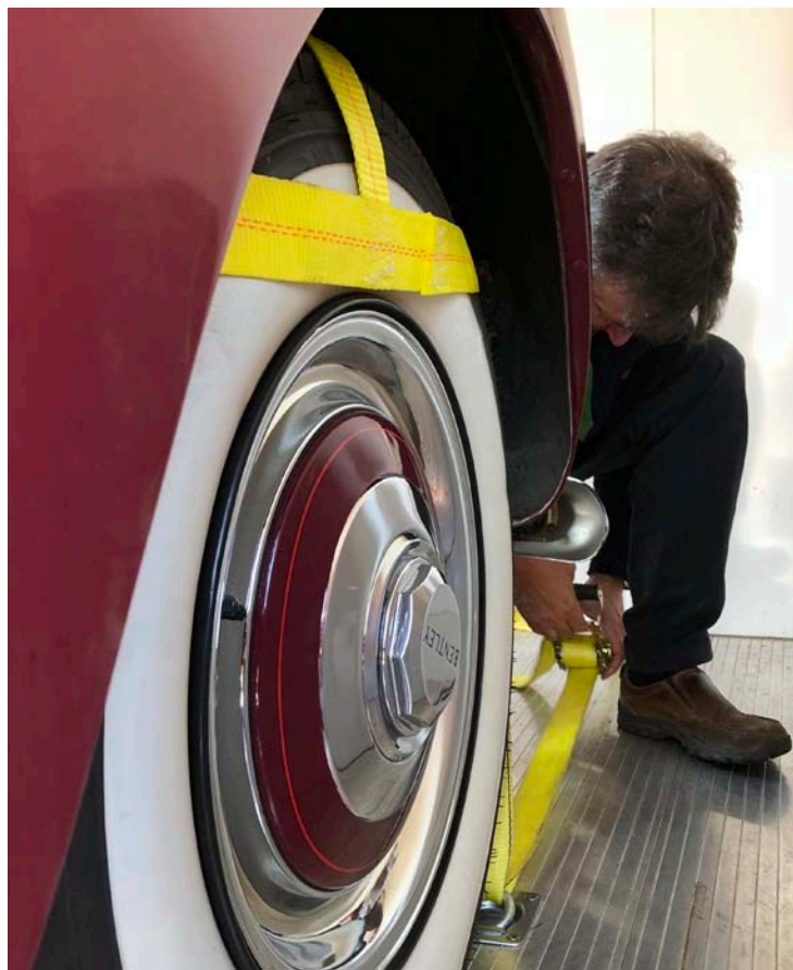
Above: The writer securing the webbing straps used on the vehicle transporter to prevent the car from shifting during its journey.
