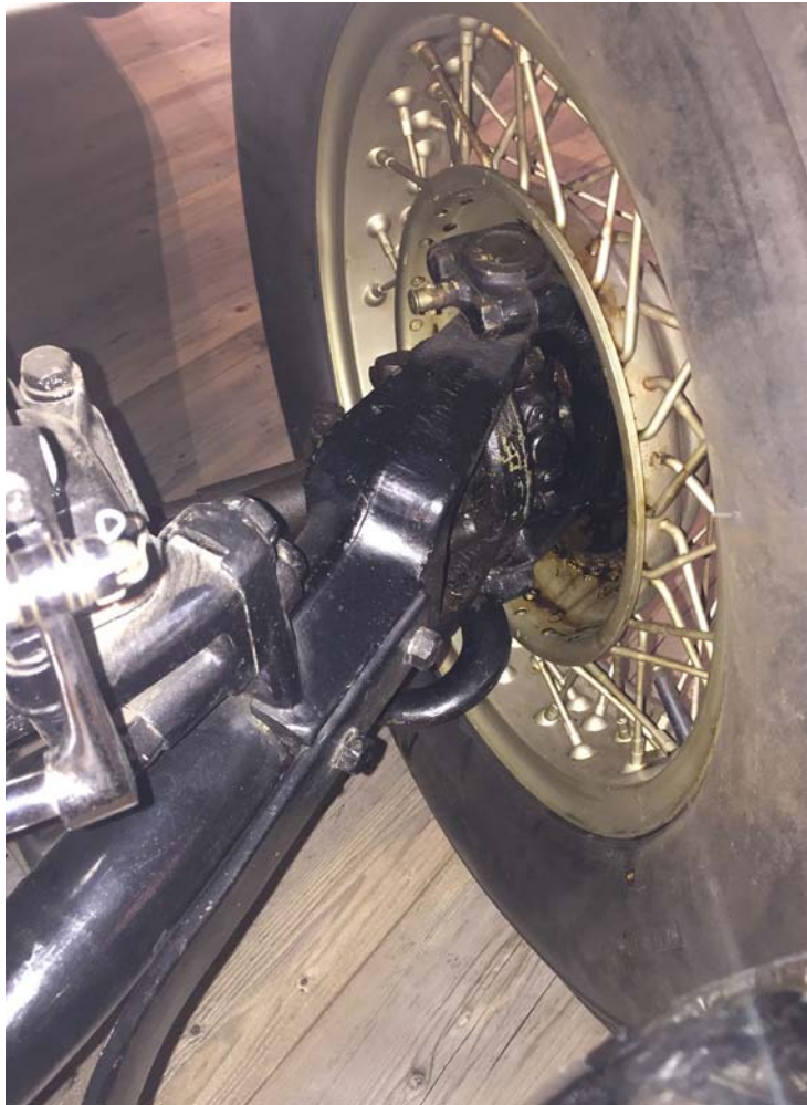
Above: The Cord front wheel drive system, 1928.
