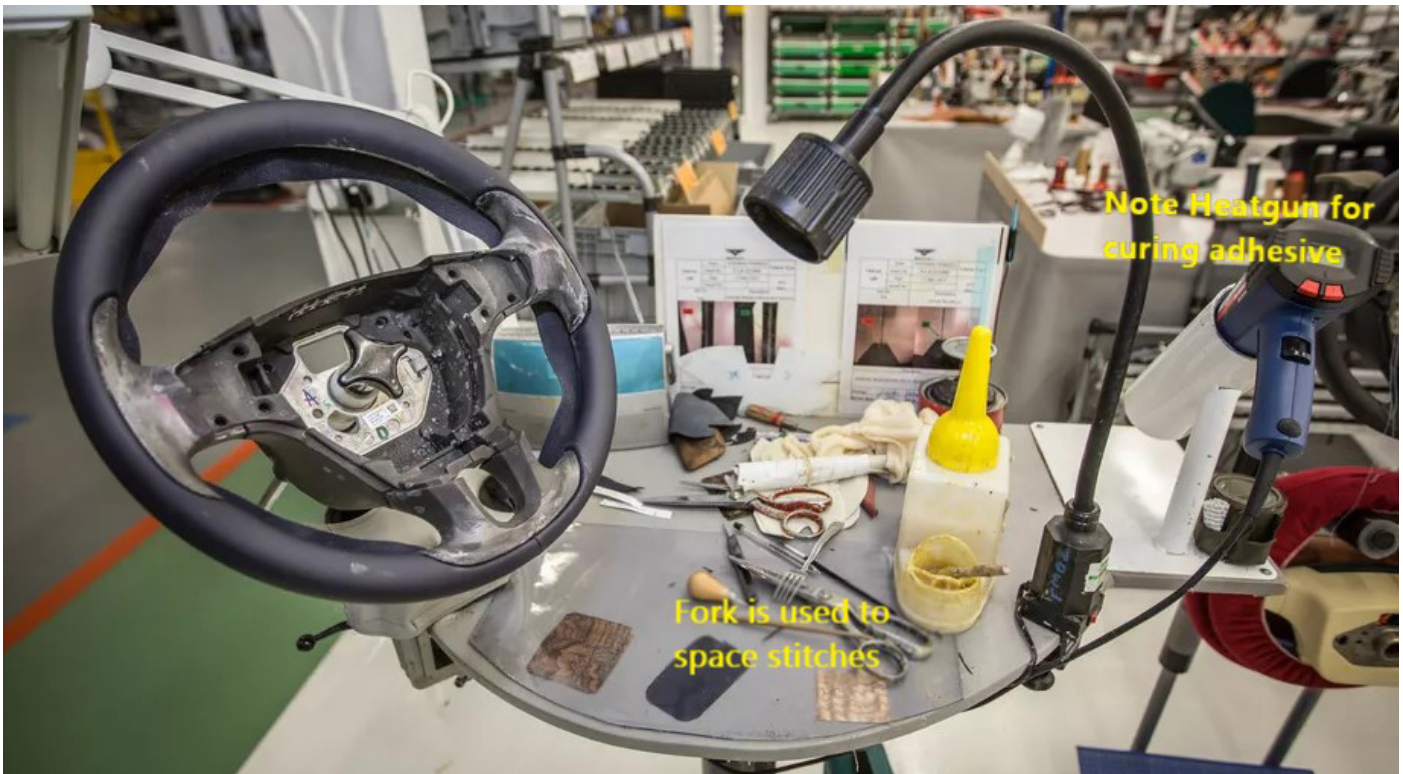
Above: It is about a 40 minute process to finish a steering wheel. Part of the show is when an operator uses a fork to mark the spacing for the stitches in the leather covering.
