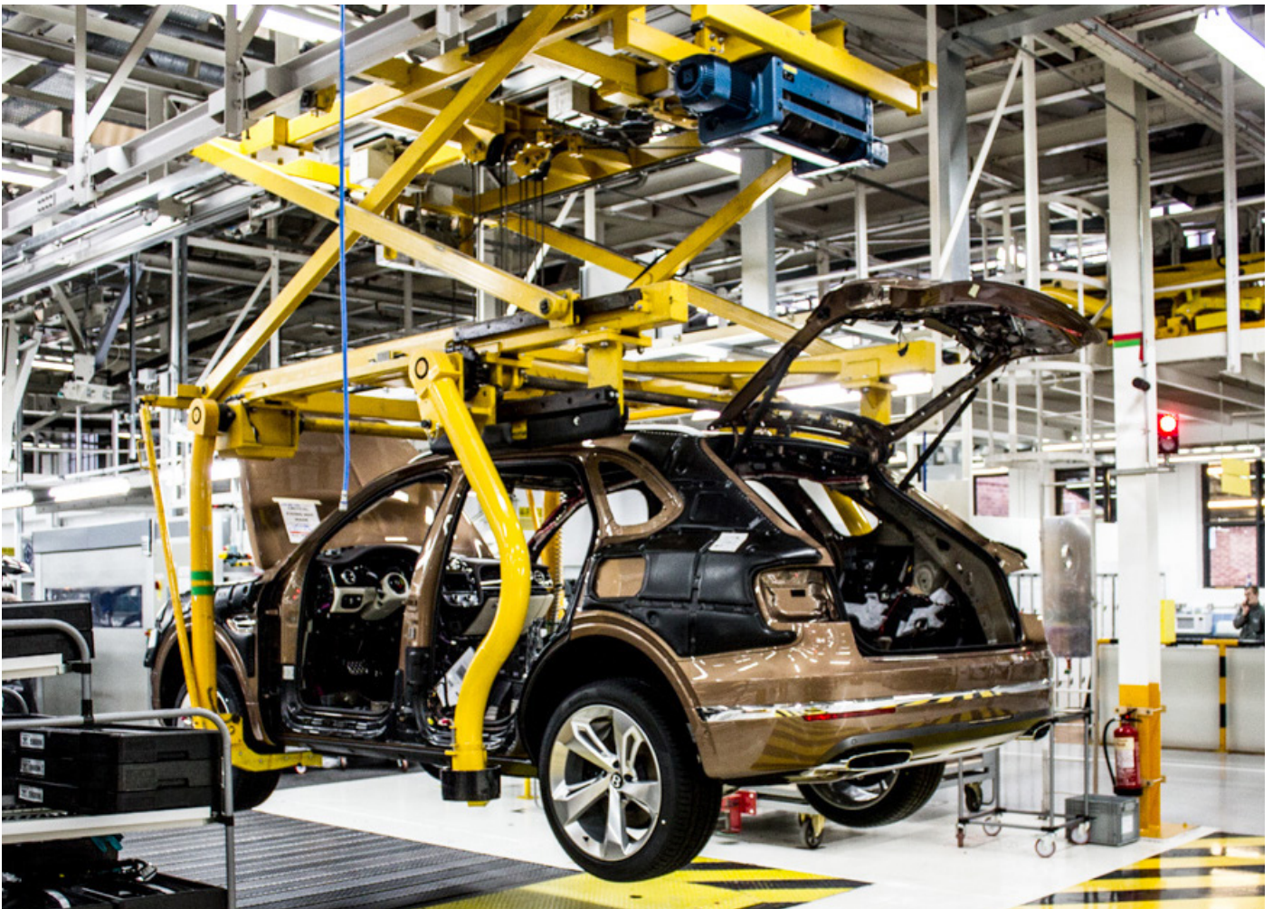
Below: The Bentayga line consists of 46 “stations”. Each assembly typically spends 16 minutes at each.
