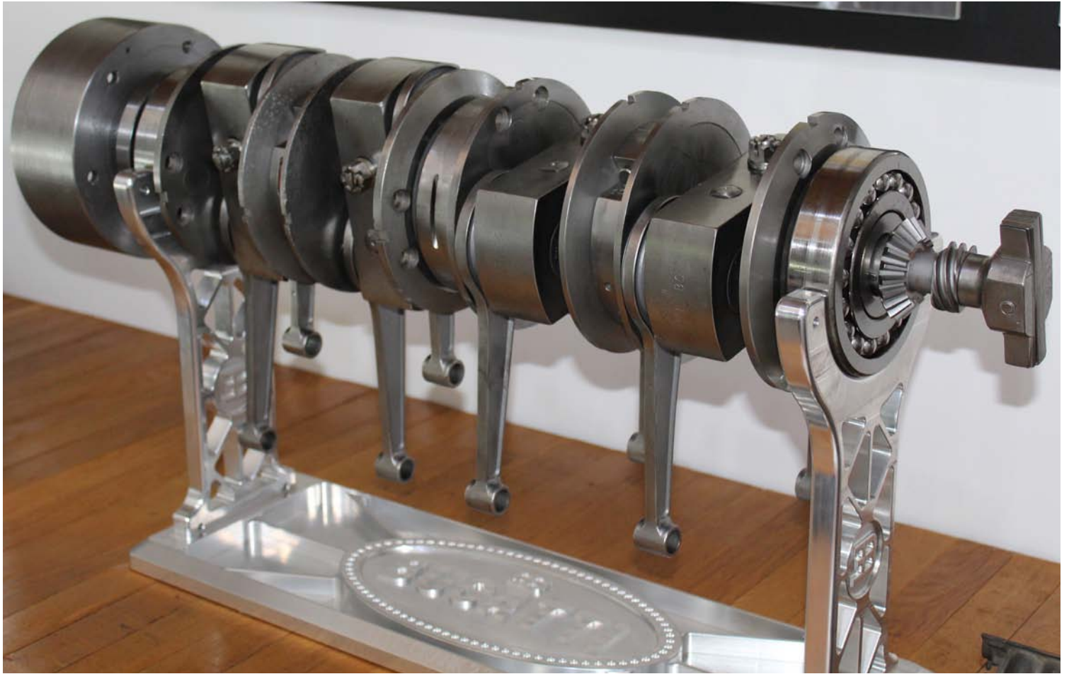
Above: The design, craftsmanship and materials in this Bugatti Type 35 straight-eight roller-bearing crankshaft inspire the greatest admiration. Note the bolts which are effectively cotter pins, locking the segments together more or less as bicycle cranks were done. Every aspect of this is superbly machined. Photographs by Gos Cory except where otherwise credited.
