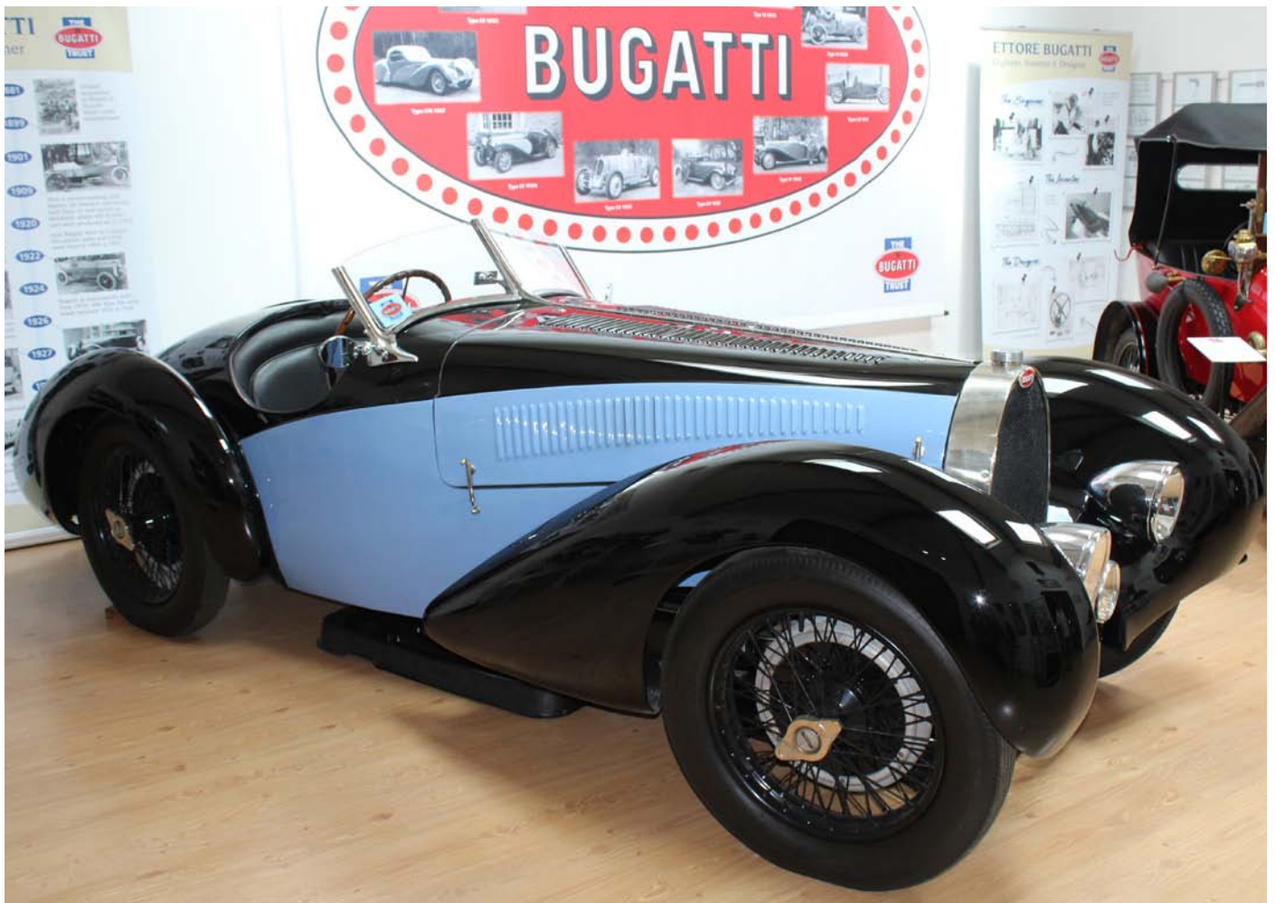
Above & below: A 1931 Bugatti fitted in the late 1930s with Paris-built (probably) coachwork, a Type 38A engine and a Fiat gearbox, then more recently a reproduction Type 51A chassis. In the background is one of Bugatti's early automotive designs, the Peugeot B  b  .
