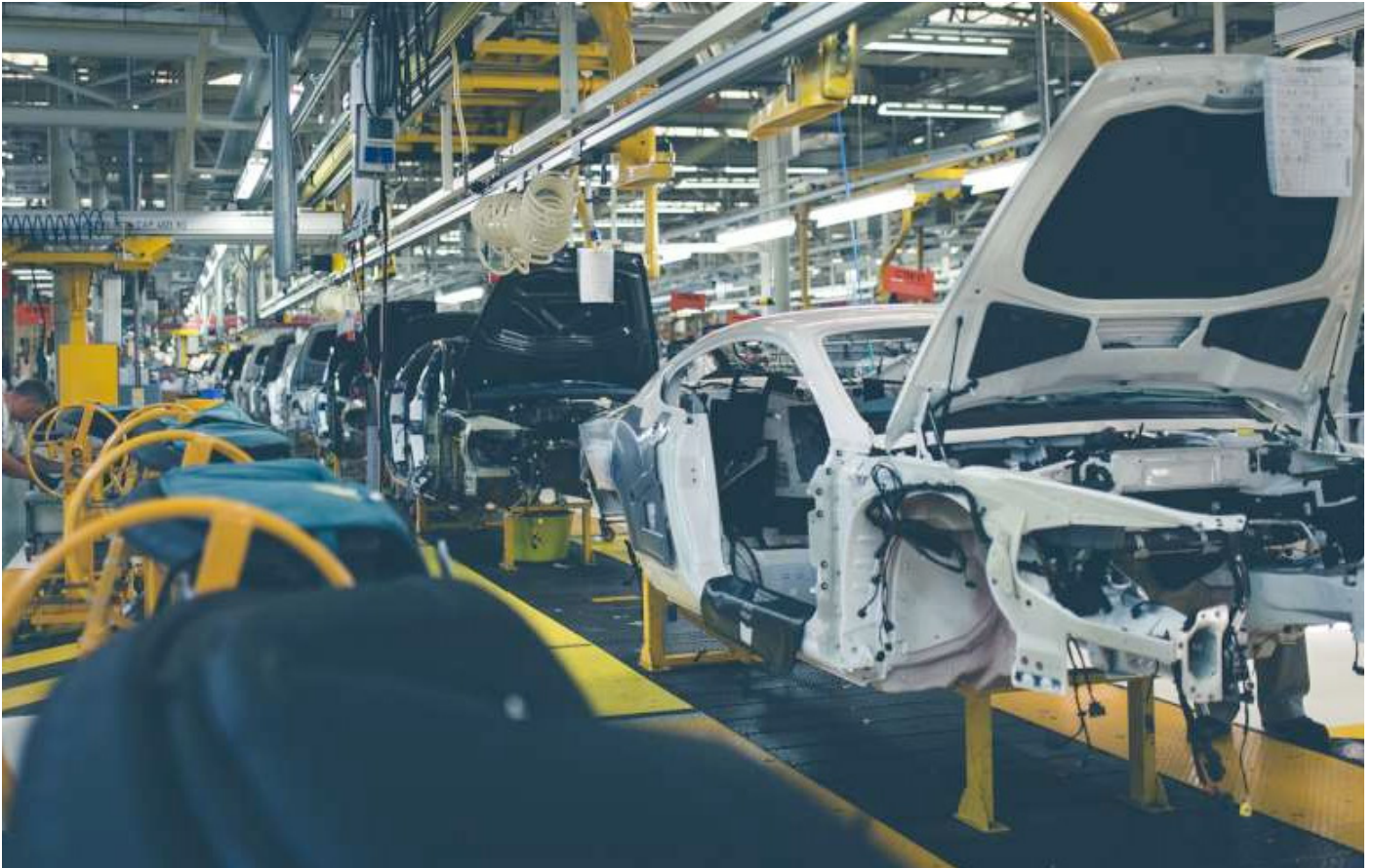
Above: The GT and Flying Spur lines consist of 68 “stations”. Typically each assembly spends 12 minutes at each. Electronic notice boards display the line speed and output targets and progress.
