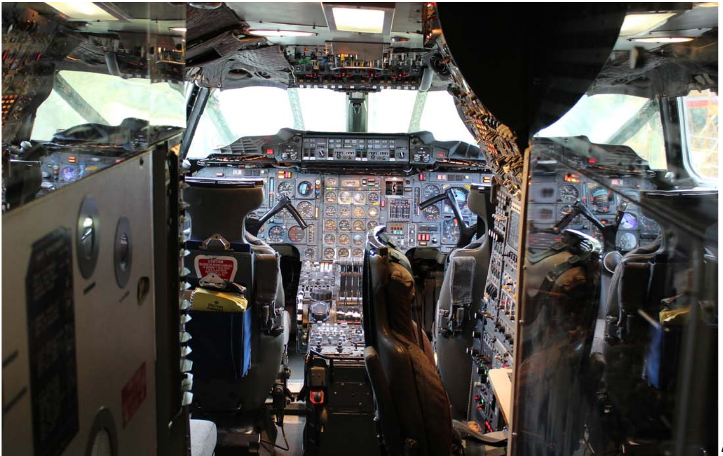
Below: The flight-deck of the prototype Rolls-Royce 'Olympus'-powered Concorde supersonic airliner. While the instrumentation looks similar to that of a sub-sonic jetliner the entire payload area is devoted to other data acquisition, cabling and additional avionics.
