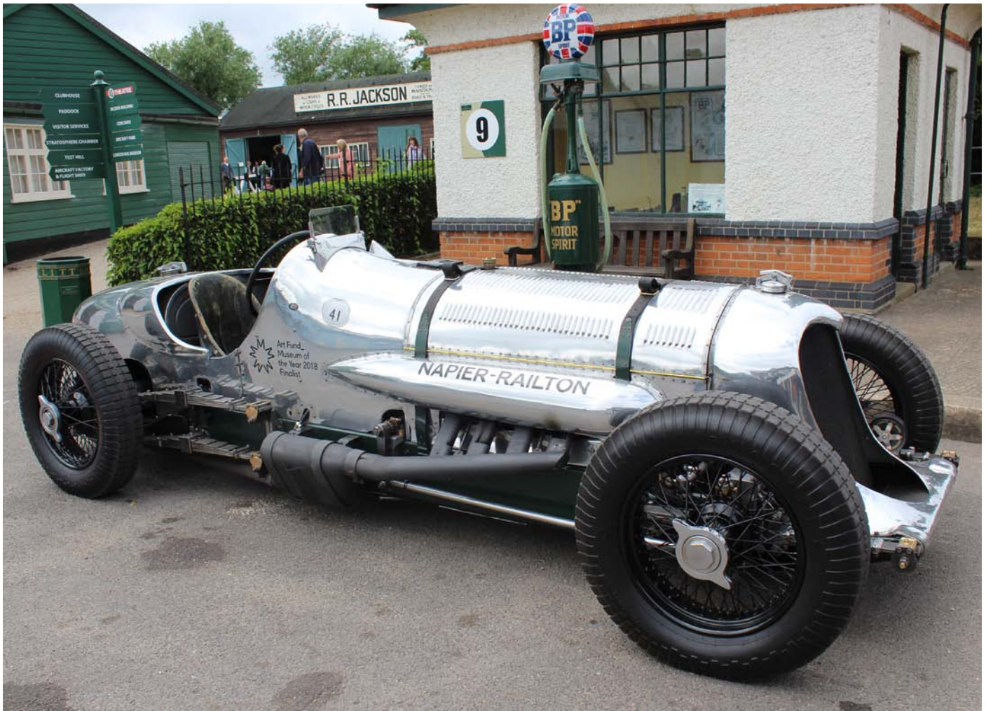
Above: 1933 Napier-Railton Special, endurance record and track racing car, commissioned by the driver John Cobb, designed by Reid Railton, powered by a 24-litre Napier aero-engine and built by Thomson & Taylor within the Brooklands Track. It achieved many Brooklands and World speed records including the Brooklands Record of 143.44 mph which was never beaten. It is owned by the Brooklands Trust. Photographs by Gos Cory except where otherwise credited.
