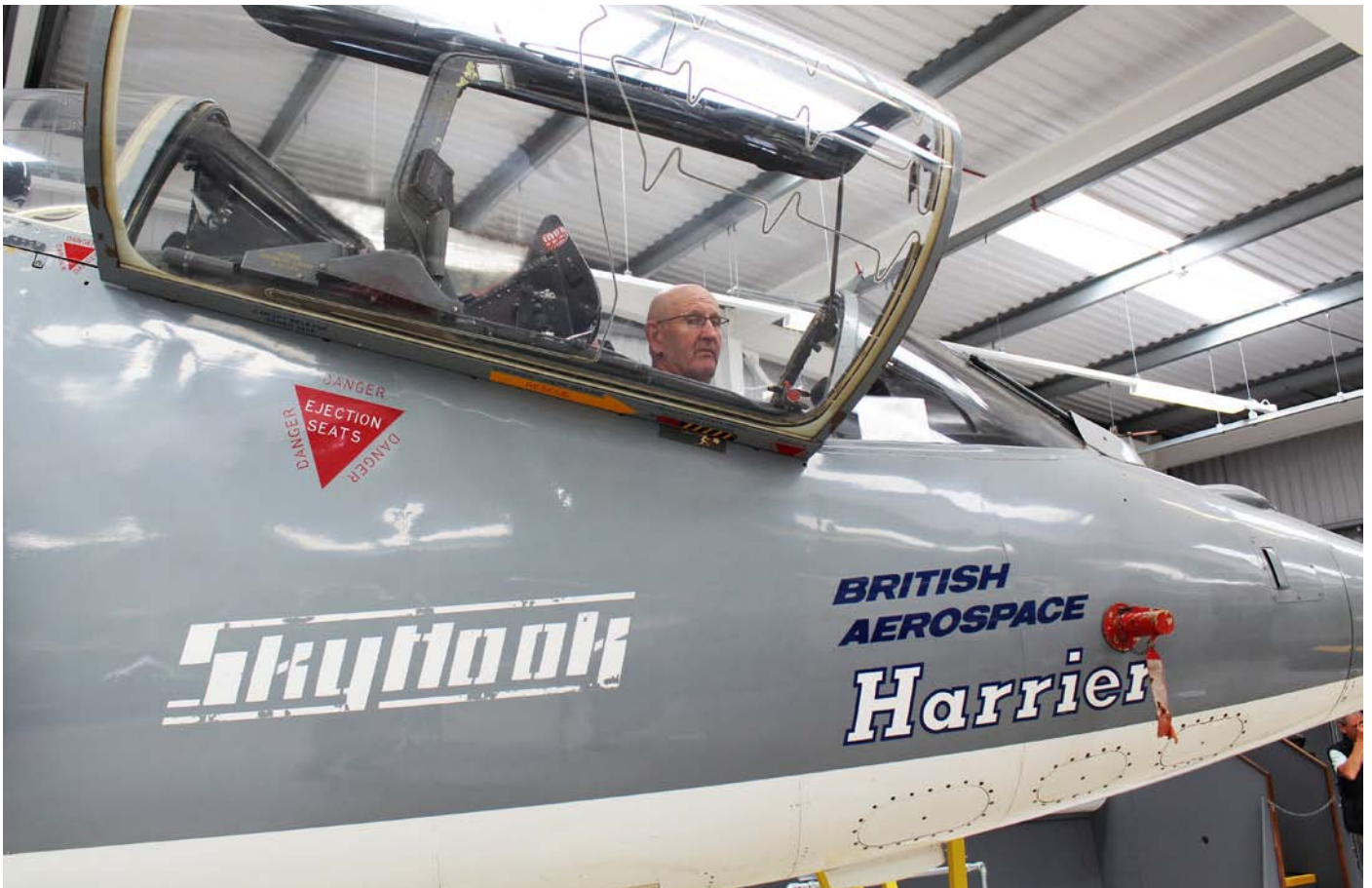
Above: Hawker Harrier T.Mk.52, 1971. The Harrier was the first successful Vertical/Short Take-Off & Landing (V/STOL) fighter, controlled by four Rolls-Royce 'Pegasus' jet engines, allowing these aircraft to take off or land almost anywhere. Visitors are able to sit in the cockpit and the writer is seen trying the pilot's seat for size. Photograph by Michael Barnes.
