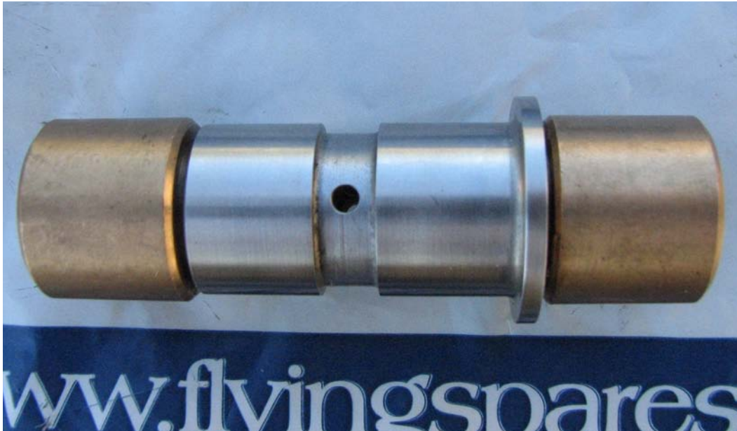
Above: The early post-war steering centre lever fulcrum pin, part number RF4075, and its bronze bushes. The ready supply of spare parts for these cars, at often more than reasonable prices, must be the envy of owners of less well-supplied marques.
