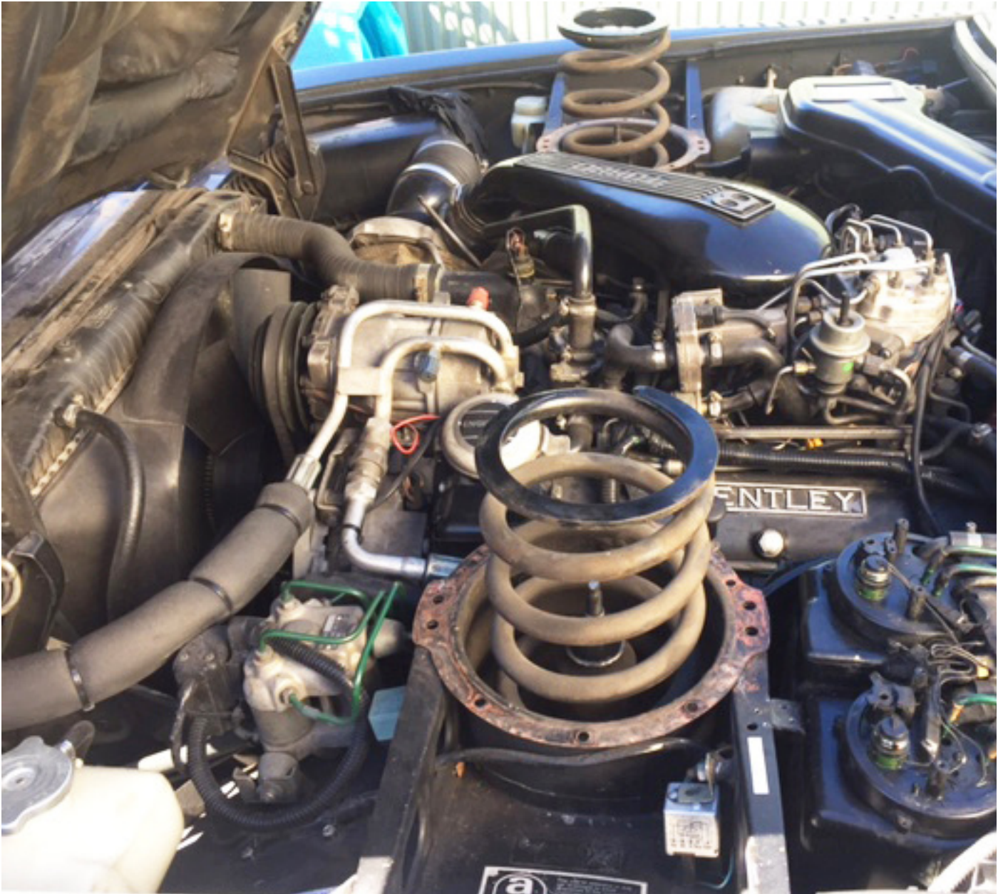
Above: Under-bonnet view with the spring top-plates removed ready for replacement. Photographs by Heather Watt.
