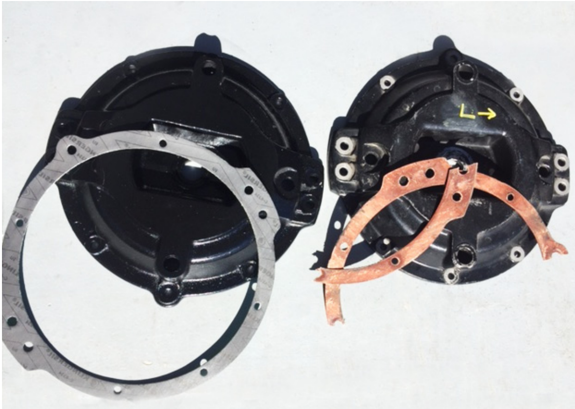
These are John Tetley's front spring top plates ( above ) and shock absorber grommets ( below ) of his Bentley Turbo R. In both photographs, the new items are on the left and the old on the right.
