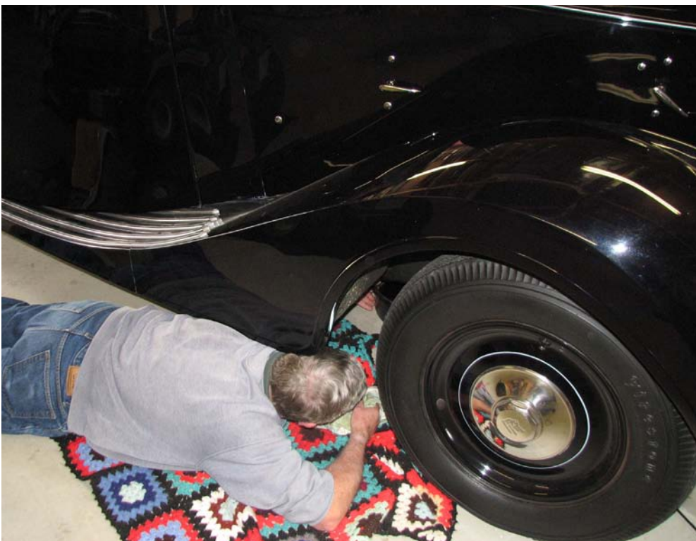
Left: The position to be adopted by the owner when removing and replacing the sump-plug of an early post-war Rolls-Royce or Bentley motor car. This is Bryce Ronning changing WFC67's engine oil.
